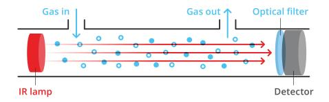
Aranet4 uses the nondispersive infrared (NDIR) sensor to measure the concentration of  $CO_2$ . The  $CO_2$  gas in the chamber absorbs infrared light and this absorption is measured by the sensor. The less light passes through – the higher the  $CO_2$  concentration. The  $CO_2$  gas absorbs only a specific wavelength of the light therefore an optical filter is used.
